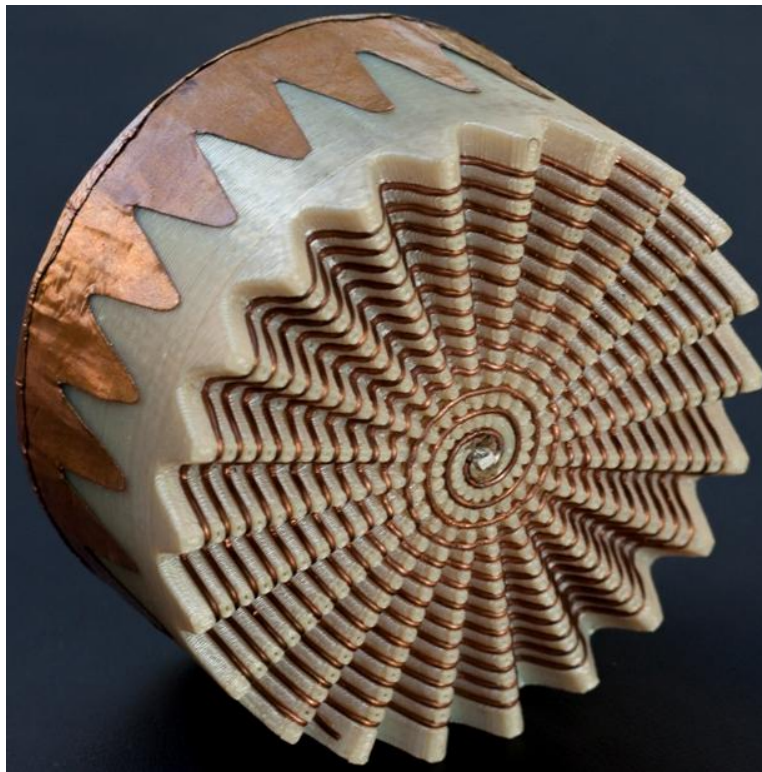
Figure 4.19: Fabricated model of sinuous cavity backed PSA antenna utilizing a linear growth profile
